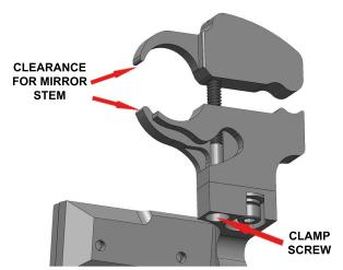
STEP 3 - BEFORE FULLY TIGHTENING THE CLAMP SCREW, POSITION THE MOUNT AS FAR FORWARD TO-WARDS THE WINDSHIELD AS YOU CAN. MAKE SURE THE TOP AND MID SECTIONS ARE TOUCHING AT THE PIVOT POINT. If you can not get them to touch at the pivot point, you have an incompatible mirror type for this mount.
