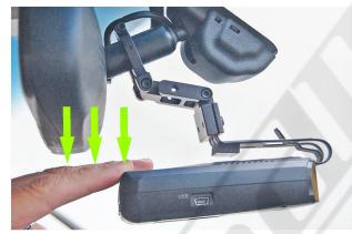
**STEP 6** - If the RD is too close to the bottom of the mirror, You may access the buttons on top of the RD by gently pushing downward on the front of the RD with one finger and push the desired button with another finger. Then allow the RD to return to it's original position by gently letting it spring upward. When accessing the buttons, be sure to push the RD downward just enough for your finger to fit between the RD and mirror. **Do not push down more than what is needed.**
